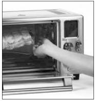
Hold the assembled Rotisserie Spit at a slight angle with the right side higher than the left side. Insert the left side of the Spit into the Rotisserie connection point inside the appliance. With the left side securely in place, drop the right side of the Spit into the Rotisserie connection point on the right side of the appliance.
